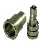
THE PATENTED DESIGN IS FOR AUTOCLAVE/OVEN WALLS AND HIGH TEMPERATURE TOOLING. THE CARTRIDGE HOLDER SCREWS TO FORM A PERMANENT CONNECTION TO THE VACUUM LINE. THE EASY TO REMOVE CARTRIDGE PLUG CAN THEN BE RESEALED OR CHANGED OVER TO MINIMISE DOWNTIME AND MAINTENTANCE. VALVES ARE FITTED WITH VITON SEALS AND ARE FULLY RESEALABLE. ALL PARTS ARE MANUFACTURED FROM STAINLESS STEEL TO GIVE LONG LIFE. MANUFACTURED TO ISO B.
