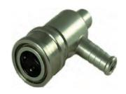
THE PATENTED DESIGN ELIMINATES THE THREADED CONNECTION PREVENTING LEAK PATHS. THE 90° HOSETAIL ALLOWS THE HOSE TO FALL AT A TIGHTER ANGLE. COUPLINGS ARE FITTED WITH VITON SEALS AND ARE FULLY RESEALABLE. ALL PARTS ARE MANUFACTURED FROM STAINLESS STEEL TO GIVE LONGEVITY. MANUFACTURED TO ISO B.
