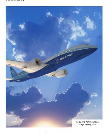
Boeing is one of the world's leading aerospace companies. The Boeing 787 Dreamliner is a long-range, mid-size, wide-body, twin-engine jet airliner. It is the company's most fuel-efficient airliner and the world's first major airliner to use composite materials as the primary material in the construction of its airframe.
