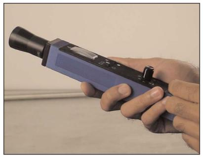
Originally designed for the US Military, the Soundscan 101 Ultrasonic Inspection System is now used in many industries throughout the world for predictive maintenance, quality control, and leak detection.
