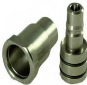
THE PATENTED DESIGN IS FOR AUTOCLAVE/OVEN WALLS AND HIGH TEMPERATURE TOOLING. THE CARTRIDGE HOLDER SCREWS TO FORM A PERMANENT CONNECTION TO THE VACUUM LINE. THE EASY TO REMOVE CARTRIDGE PLUG CAN THEN BE RESEALED OR CHANGED OVER TO MINIMISE DOWNTIME AND MAINTENANCE. VALVES ARE FITTED WITH VITON SEALS AND ARE FULLY RESEALABLE. ALL PARTS ARE MANUFACTURED FROM STAINLESS STEEL TO GIVE LONG LIFE. MANUFACTURED TO ISO B.
