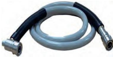
PREMIER HIGH TEMPERATURE VACUUM HOSE ASSEMBLIES ARE MADE FROM PLATINUM CURED SILICONE HOSE (GIVES OFF NO FREE SILICONE PARTICLES) AND ARE FITTED WITH PREMIER STAINLESS STEEL COUPLINGS. THE THREADLESS SYSTEMS PROVIDES THE HIGHEST VACUUM PERFORMANCE AND MAXIMUM FLEXIBILITY. ASSEMBLIES ARE FITTED WITH INTERNAL AND EXTERNAL SUPPORT SPRINGS. VITON SEALS AND ARE FULLY RESEALABLE. MANUFACTURED TO ISO B.
