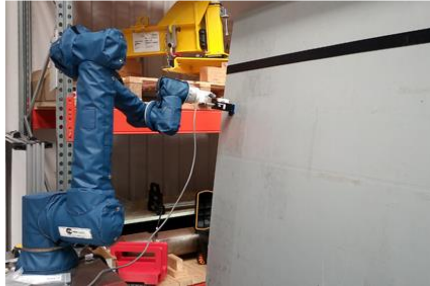
Evotis tap tester mounted on a UR10e Collaborative Robot for automated inspection of a large GFRP sample
