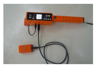
When used in conjunction with a PC a colour tile map of the area under test is displayed. A record can be saved / printed creating traceability of a scan.
