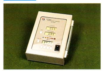
This monitoring unit when connected to WP632, shows the measured values both digitally and in a bar-graph, and memorizes them. It is provided with a connector for data transmission to a personal computer available on the market.
